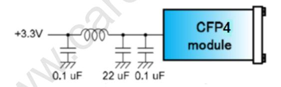
Figure 4. Recommended Power Supply Filter
